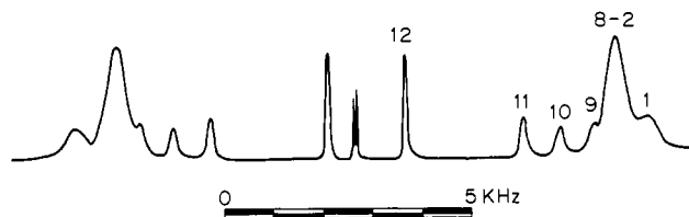
Figure 1. Deuterium magnetic resonance spectrum of type II DM mesophase prepared from the pure host detergent dodecylammonium chloride. The mesophase composition is recorded in Table I. The high-field spectrum is assigned according to the carbon segment in the chain. Extensive overlap occurs for positions 2–8 because of a long plateau of order in the profile. Since the shortest guest added is the octyl chain, the positions which are important, 9–12, do show a clean resolution on the dodecyl chain. The sharp doublet at the center of the spectrum belongs to the DOH signal.
